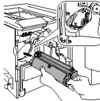
**Caution:** Do not hold a toner cartridge vertically, or touch the toner roller surface. This can result in lower image quality. If you have changed the printer cartridge you must let the calibration cycle complete (150 sec. approx.) before opening the door. You must wait for the **Ready** indicator to light up. Always install each toner cartridge in the slot of the same color.
