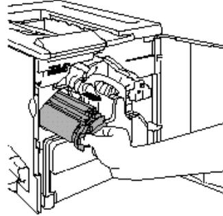
6. Before installing the new toner cartridge remove the protective cover clearly marked **REMOVE**. Insert the cartridge while supporting the middle section with your left hand. Insert the toner so that it fits into the rails in the compartment in the carousel and close the door.
